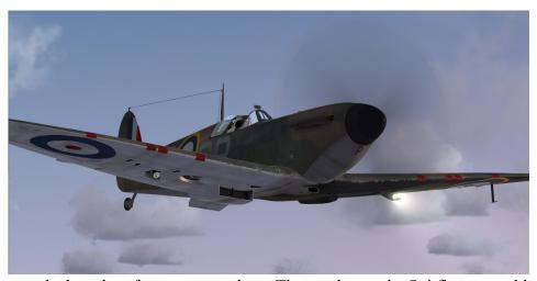
envisioned a light, maneuverable craft with low drag, elliptical wings, and a broad performance envelope. The result was the Spitfire, a capable, lethal, yet forgiving aircraft that ultimately proved more than equal to anything the Germans could throw at it, including the vaunted Focke-Wulf 190.
