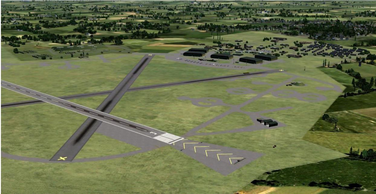
One of the last batch of pre-war expansion scheme airfields, RAF Binbrook (ICAO ID: EGXB) was built on Ash Hill in the Lincolnshire Wolds. The usual arrangement of the later Type C hangars, five in number, facing the bombing circle was backed by the administration, technical and barracks sites.
