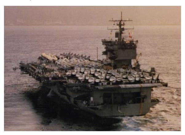
At 1,123 ft, she is the longest naval vessel in the world. Her 93,284 long tons displacement ranks her as the 11th-heaviest super carrier, after the 10 carriers of the Nimitz class. Enterprise was meant to be the first of a class of six, but construction costs ballooned and the remaining vessels were never laid down. Powered by eight Westinghouse A2W reactors,
