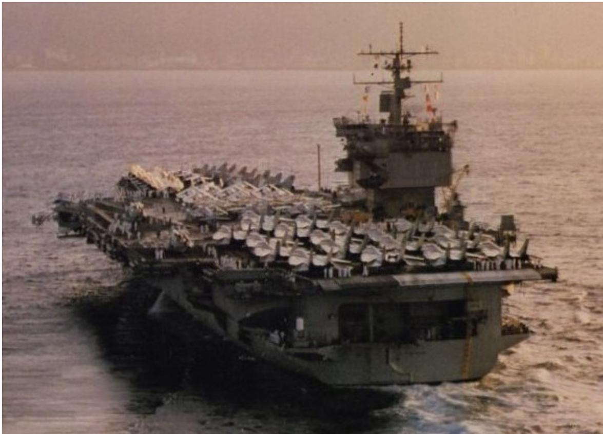
At 1,123 ft, she is the longest naval vessel in the world. Her 93,284 long tons displacement ranks her as the 11th-heaviest super carrier, after the 10 carriers of the Nimitz class. Enterprise was meant to be the first of a class of six, but construction costs ballooned and the
