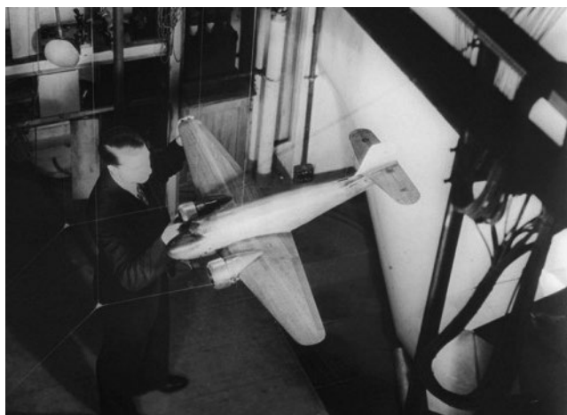
Clarence "Kelley" Johnson with the 55" scale wind tunnel model of the first, single tail design for Lockheed's Model 10 Electra.
