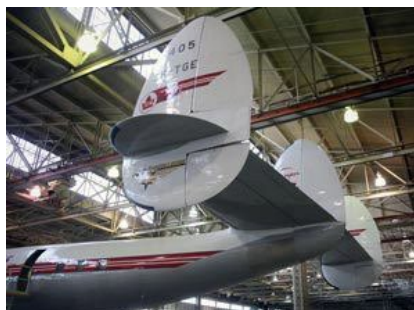
This photo clearly shows how Constellation's outer fins/rudders are mounted inboard of the horizontal stabilizers' tip.
