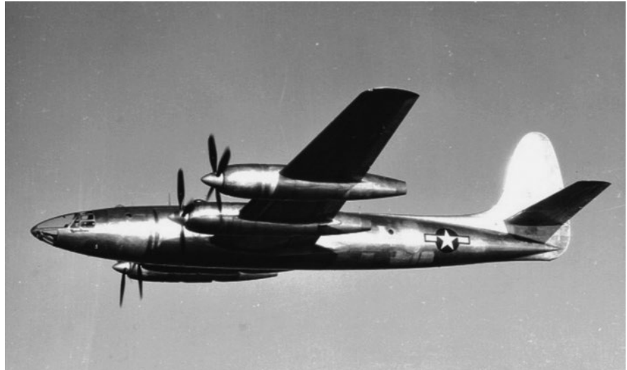
Republic "Rainbow" in the markings of the U. S. Army Air Force shortly before it became the independent U. S. Air Force. Proposed as a reconnaissance/aerial photography aircraft, "Rainbow" (USAAF designated XF-12, USAF designated XR-12) it had a top airspeed of over 470 mph at 45,000', making it one of the fastest piston-engine aeroplanes in the USAAF's inventory. However, the prototype's first problematic flight was not until 10 July 1947 when even faster jet-powered aircraft such as RB-47 were already being used for this mission. Accordingly, none were ordered and only two were built. Quel dommage, it certainly is a beauty.
