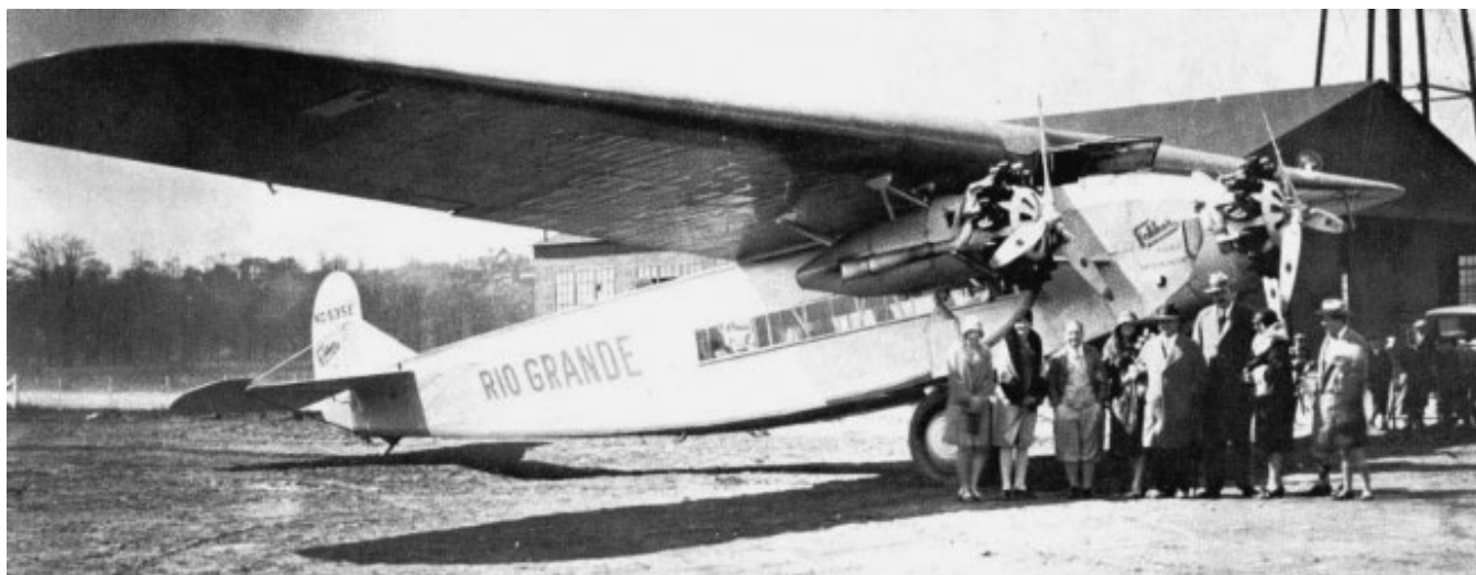
1928 Fokker F. 10A, was an improved and more powerful F.10. It had three 425 hp Pratt and Whitney Wasp C radial engines and carried up to twelve passengers, but only eight well-to-do looking passengers appear to be about to board when this photograph was taken. Note the thick, cantilever, plywood-covered wing, the drag-producing, exposed engines and the W.W.I Fokker fighter-style fin and rudder.
