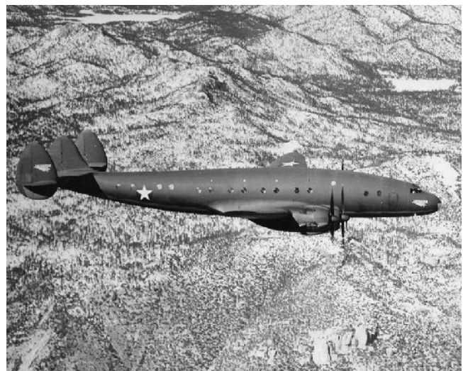
This is the first USAAF Lockheed XC-69 prototype, which had its first flight on 9 January 1943. It is easily identified as such because it is reliably reported that it was painted in full USAAF camo (Olive Drab 41 on top, Neutral Grey underneath), had the white star in blue circle with no red centre circle insignia, no Army serial numbers on the tail, and most unusually, large Lockheed logos on the tail and nose. This C-69 was a USAAF aeroplane at this time and as such would not ordinarily be marked with civilian factory logos, especially not so prominently.
