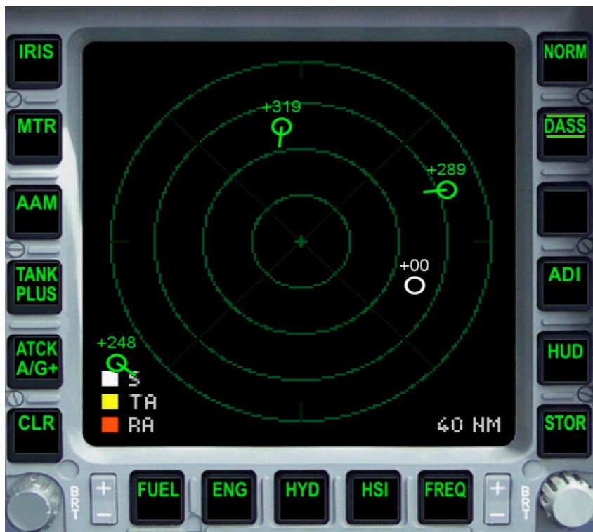
„DASS“ – Defensive Aids Sub System – automatic air surveillance here AI-traffic radar 30 NM
