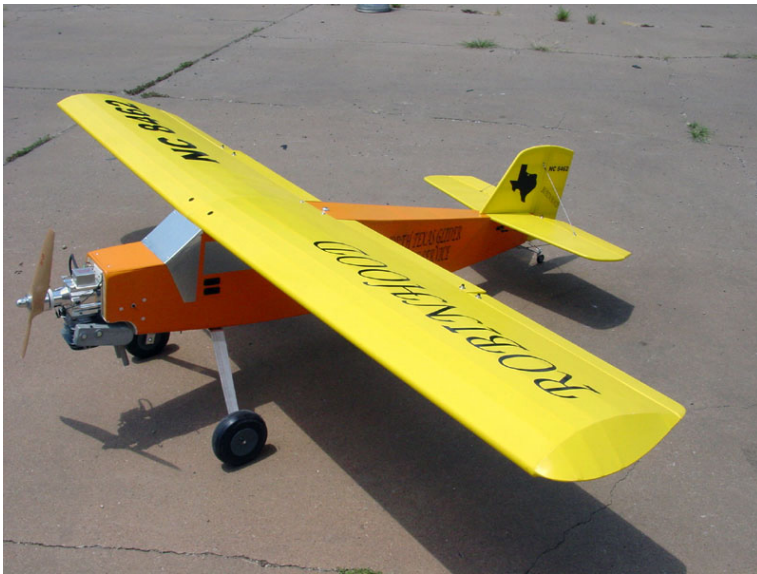
Radio controlled Curtiss Robin model popular for sailplane towing. Note the average aspect ratio of the wing.
