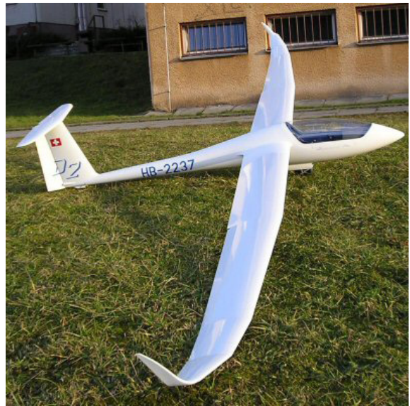
5- Metre Discus R/C sailplane. Note the extremely high aspect ratio of the wing.
