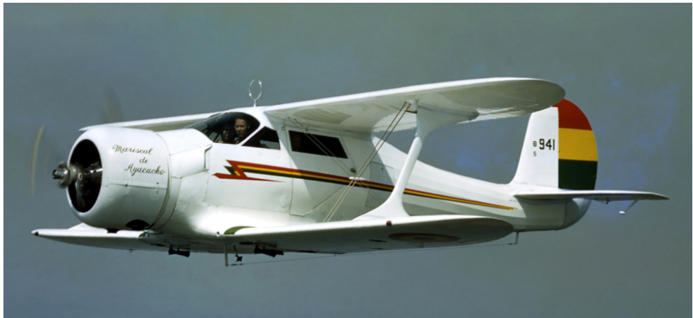
A beautifully restored Belgian-registered Beech Model 17S “Staggerwing.” This unique and striking design is a massive and complicated fabric-covered wood and steel structure powered by a 450 hp Pratt & Whitney R-985-AN-1 “Wasp Junior” radial engine. With a top airspeed of 212 mph (184 knots, 341 km/h,) it was a fast biplane in the 1930s, but became less and less competitive as an executive transport with the emergence of the new and more efficient all-metal aviation technology of the 1940s.
