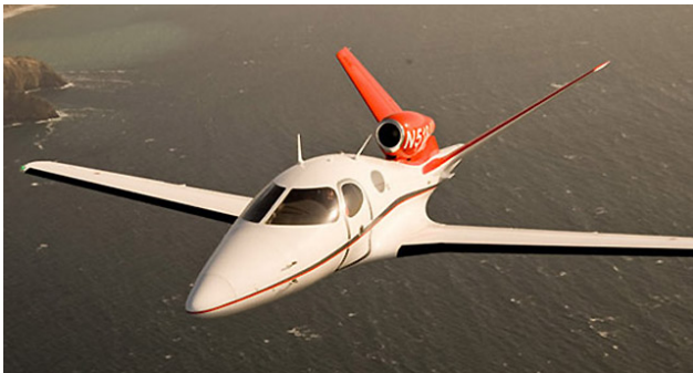
■ Eclipse Aviation 400. If you're going to put a single jet engine on top of the fuselage a "V"-tail seems like your best, if not your only bet.
