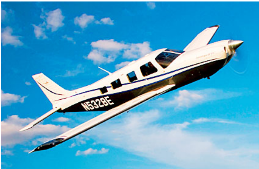
Piper PA-32R "Saratoga." This advanced and very high-performance aeroplane was initially called "Piper Lance," a retractable undercarriage Piper PA-32 Cherokee Six. As this aeroplane evolved it became known as Piper "Saratoga." Similar to Lance in most ways, Saratoga has a tapered wing, whilst Lance's wing is Cherokee Six's un-tapered "Hershey Bar" type.
