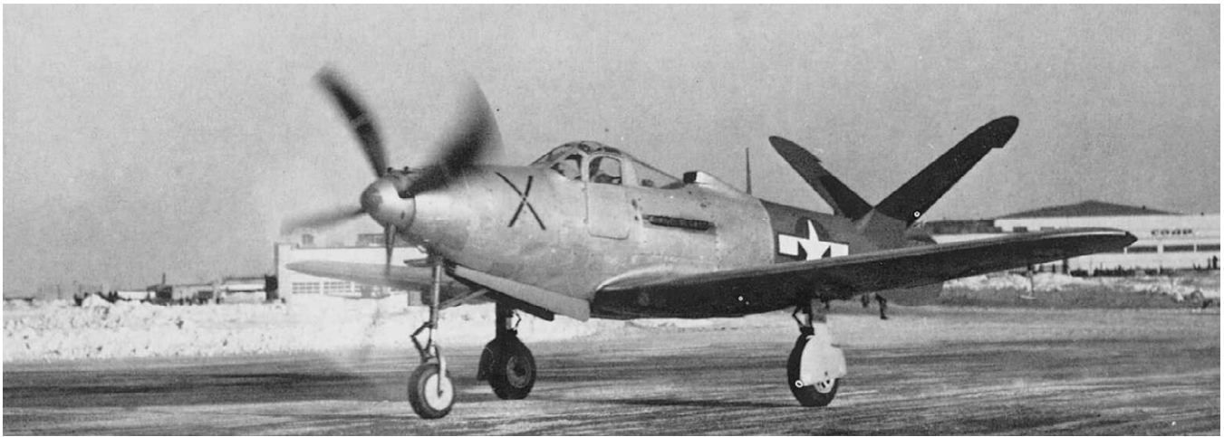
1944 Beech built a one-off A-19, which was a USAAF A-10 "Wichita" with an experimental "V"-tail. A-19 was the first and largest Beech aircraft to that date with such. At the time, many might have wondered why Beech was experimenting with a "V"-tail. Time would soon solve that mystery. A-19 would certainly be a challenging subject for a "can you name this aeroplane" contest. USAAF archive photo, circa 1944.
