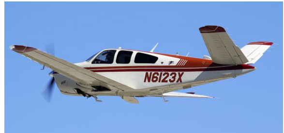
Beechcraft Bonanza V35B – a study in grace and power. The last “V”-tail Bonanza, not at all coincidentally designated V35 was introduced in 1966. Minor improvements to it were made in V35A (1968-69) and many more in V35B (1970-82.)
