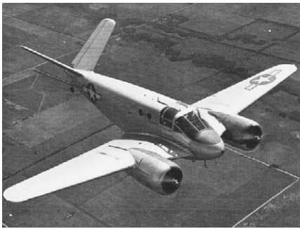
1944 Beech built a one-off A-19, which was a USAAF A-10 "Wichita" with an experimental "V"-tail. A-19 was the first and largest Beech aircraft to that date with such. At the time, many might have wondered why Beech was experimenting with a "V"-tail. Time would soon solve that mystery. A-19 would certainly be a challenging subject for a "can you name this aeroplane" contest. USAAF archive photo, circa 1944.
