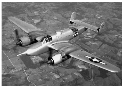
■ The second and last prototype Beechcraft XA-38 “Grizzly” shown here was produced with an operational 75 mm cannon. It beggars one’s imagination to think that the same company which was still producing the fabric-covered “Staggerwing” biplane also designed and built this formidable-looking and performing modern warplane. Photo from “Old Machine Press”
