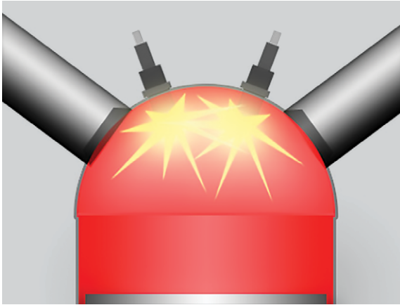
The air and fuel are compressed by the piston, then the ignition system adds the spark to create a controlled explosion.
