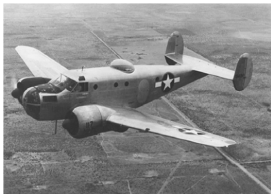
■ Beech AT-11 “Kansan” bomber trainer over Texas in 1943. One of 49 military variants of Model 18, AT-11 was the U. S. Army Air Force’s (USAAF) primary bombing trainer during the war in which more than 40,000 bombardiers were trained. Modifications included a transparent bomber’s nose, an internal bomb bay and bomb racks and a dorsal gun turret for gunnery training. Photo from “Western Trips”
